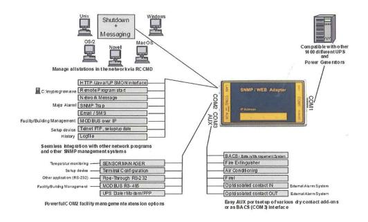
Note: The "CS121 BUDGET" is an economic version of CS121 has no COM2 (for sensors, modbus, modem, Pipe-Thru, terminalconfiguration) and AUX (dry contact and BACS interface). Beside this the BUDGET is identical to the full-qualified CS121.
